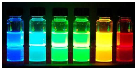
Figure 2.6: Photoluminescence of alloyed \text{CdS}_x\text{Se}_{1-x}/\text{ZnS} quantum dots of 6nm diameter. 7 As the composition of the \text{CdS}_x\text{Se}_{1-x} alloy is changed, so is the photonic emission of the dot.
